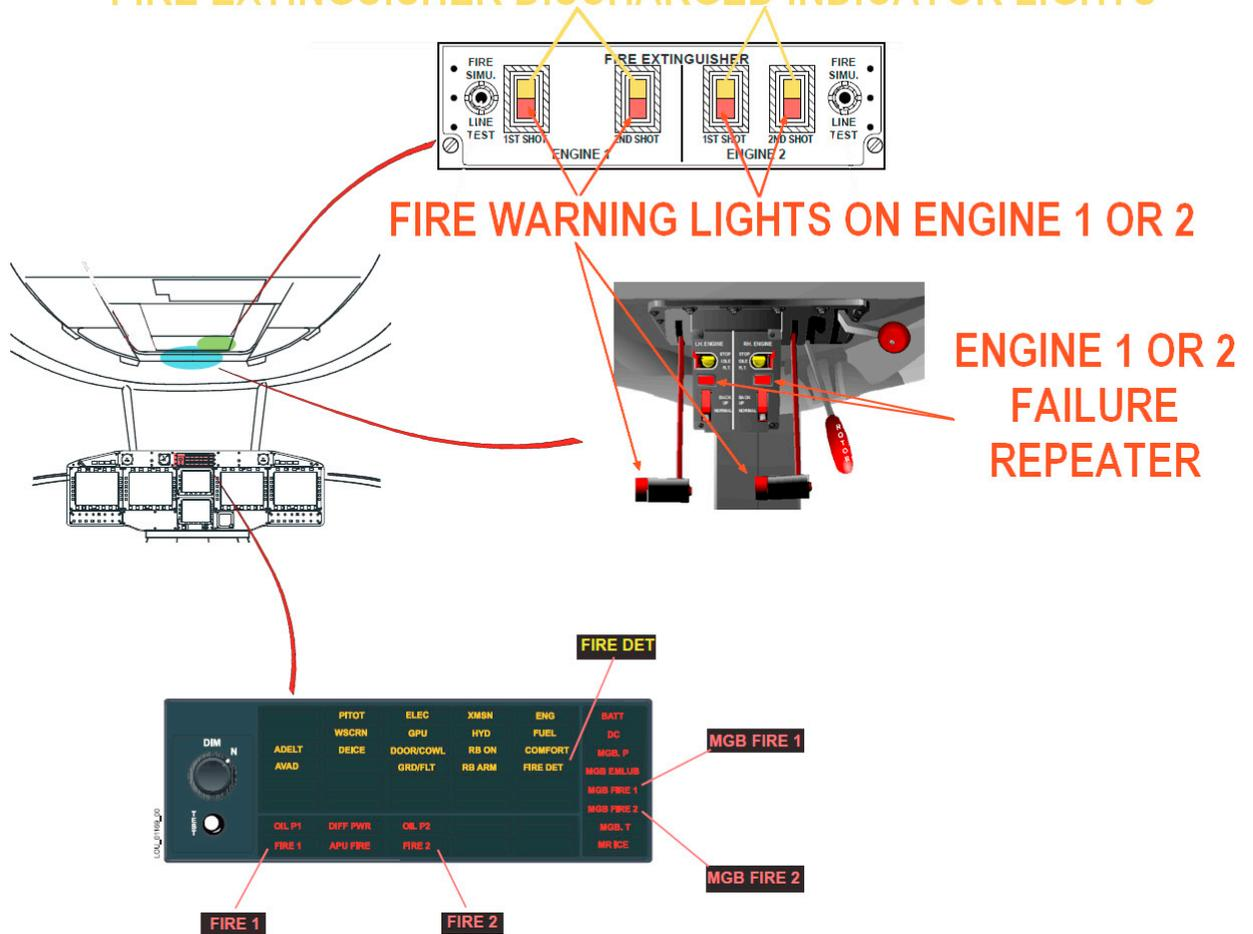
**PROCEDURE IN CASE OF ENGINE FIRE DETECTION**
