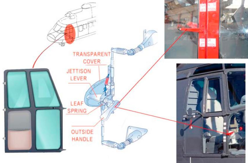
Doors can be jettisoned by actuating the jettison lever, secured by a leaf spring and protected by a breakable transparent cover. It causes the door to fall away. It can be operated from the outside by the outside handle.
