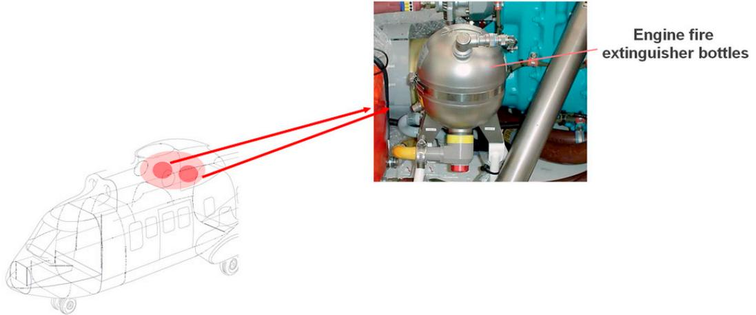
The system consists of detection and extinguishing circuits with two Halon fire extinguishers.
