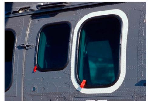
Fixed windows (including the ones of the sliding doors) are jettisonable from inside or outside by pushing out strongly after removing the seal-retaining strip.
