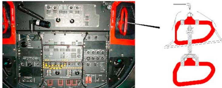
Actuating one general CUT-OUT handles shuts off both engines and cuts off all the electrical supplies except the engine fire extinguishing systems and some necessary items (triple NR indicator...).
