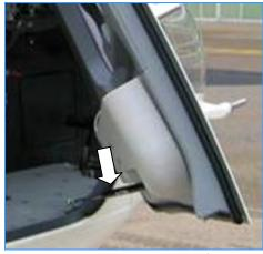
To enlarge the door opening, unhook the gas pressure spring by pressing it upward with some force on the cabin side.
