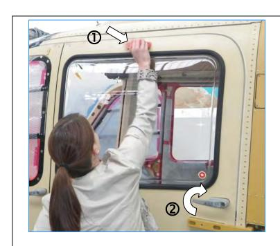
1: **Pull** emergency handle 2: **Turn** door handle **at least** 90°, then **pull** the sliding door **outwards**
