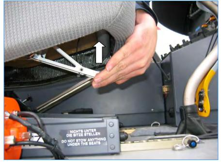
Pull the lever under the seat to move the seat forward/backward
