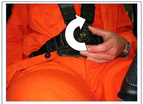
To open the safety belt, press the turn lock until each belt is free.
